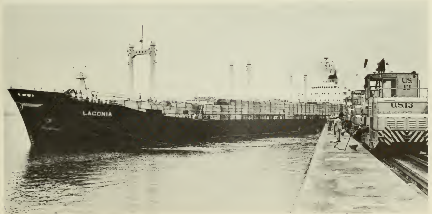
The Laconia, guided by the radio communication between the locomotive operators and the pilot on board, enters the locks.
